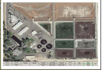
**7. Justification & Useful Life:** Depending on sludge volume index and desired margin of safety (mean cell resident's time, nitrification and denitrification), the plant is about 94% of capacity with aeration basin 3 only. Aeration basin 3 is the prime use basin. As flows and loadings increase Aeration Basin 2 will need to be placed into service.
